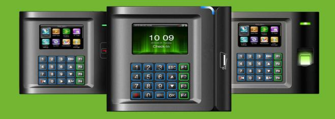
US15C-R / US15C-B / US15C-M / US15C-ID is an innovative standalone RFID / barcode / magnetic stripe / Fingerprint time and attendance reader. With a color 3 inch TFT display, offering unparalleled performance on an embedded Linux platform with all the features of a modern time and attendance reader.
